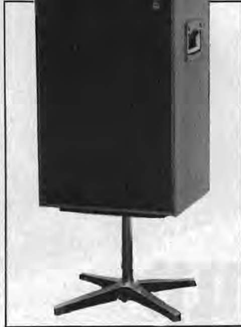
Chartwell PM450P, a polypropylene drivered, high efficiency enclosure related to the LS5/8. The electronic version contains an active crossover and a Quad 405 power amplifier feeding a full 100 watts to the 12 inch bass driver and an attenuated 12 watts to the large diameter soft-dome tweeter.
