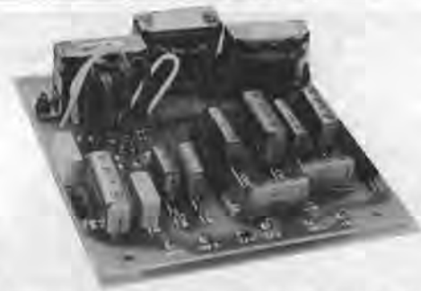
Eighteen element crossover board for the LS3/5A enclosure, the seven position tap can be seen in front of the autotransformer at the back left of the board.
