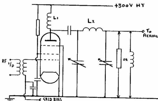
The "+300V" is connected to the anode via inductance L1 which will pass the anode current but block the Radio Frequency.
