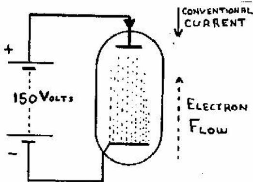
Thus, with the *High Tension battery* connected as shown there will be a strong stream of electrons flowing, across the vacuum, from Cathode to Anode. If, however, the battery were turned round, the then negative Anode would repel the negative electrons and the flow would cease.
