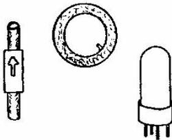
Mention a valve and you are likely to think a 'non return' item of plumbing or the little things on your car tyre to connect the air 1 Inc to. There is an important similarity with the Radio Thermionic Valve... they all allow flow in one direction only, be it water, air or in our case - electrons.
