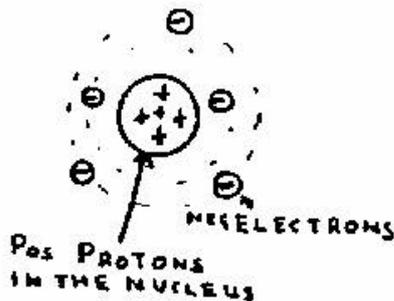
An atom comprises: a central Nucleus and a number of orbiting negatively charged Electrons. The Nucleus is made up of positively charged Protons and perhaps some uncharged Neutrons. Normally, the number of protons is equal to the number of electrons.
