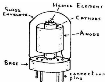
By heating the metal (called the cathode) the electrons become very agitated and many of the electrons escape from its surface.
