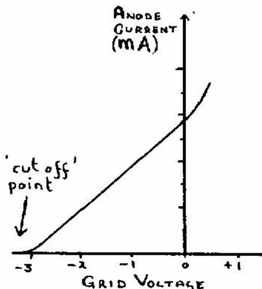
If the grid is not connected to anything, it won't have any effect. However, a small negative voltage on the grid will make a difference. The negative grid will repel some of the negative electrons and therefore cut down their flow from Cathode to Anode. The actual effect on the flow depends on the size of the negative voltage (grid bias) as can be seen, in the graph on the left. It shows the relationship between the negative grid bias and the Anode current.
