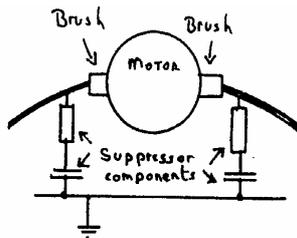
It was soon recognized that such interference was antisocial. However, it was quite easily avoided - each motor was manufactured with a suppressor" fitted. This damped the spark and greatly reduced its annoying radiation. The circuit, although simple, was generally effective. Add-on suppressors then became available to fit to earlier un-suppressed motors.
